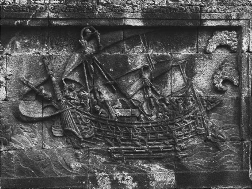
This bas-relief shows that outriggers, square sails, and rear-mounted rudders were all employed on medium-sized ships in insular Southeast Asia. This image is on the port side of the ship at the eighth-century Borobudur stupa in central Java, Indonesia. Mararie, “Ship Relief,” September 18, 2012. Photo courtesy of Marieke Kuijjer
